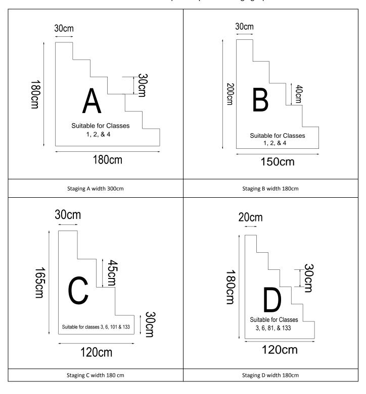
All staging is constructed of rough sawn timber.
